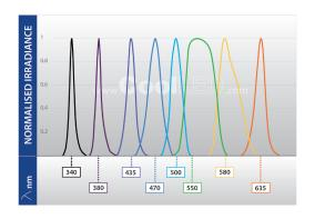
**Fluorescence Freedom:** 8 powerful LEDs span 340-635 nm to cover all popular calcium and pH indicators, fluorophores and opsins from Fura-2 to Cy5, as well as novel fluorophores which become available in the future.
